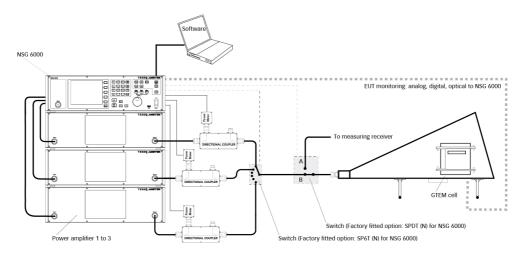
Example of test setup 9 kHz to 6 GHz with three power amplifiers and measuring receiver
