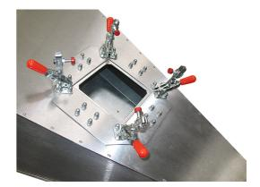
GTEM 250A-SAE with view to opening for IC testing, on the left with cover plate
